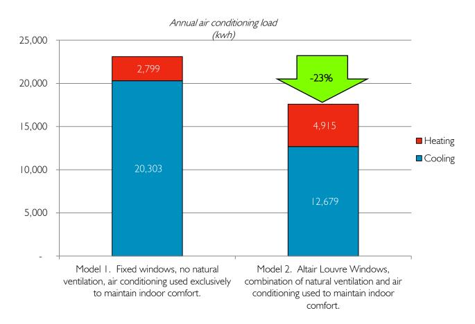
The results of this independent modelling study show that the energy reductions due to the use of Altair Louvre Windows that enable cooling natural ventilation far outweigh the reductions in air conditioner efficiency due to the air infiltration rate of the Altair Louvre Windows.
