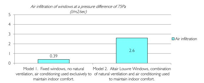
Note: The air infiltration of the fixed window is the average air infiltration rating sourced from www.wers.net of 9 different fixed windows from 4 different manufacturers,
