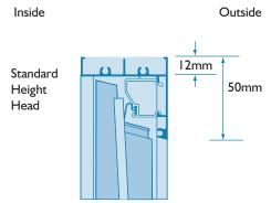
Example shows the Glass / Aluminium Fixed Blade Carrier. A Timber Fixed Blade Carrier is also available.
